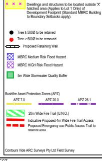
Indicates Development Footprint Area to contain all dwellings, structures, on site stormwater drainage, on site parking, driveways, access and manoeuvring areas, on site wastewater treatment systems. Effuent disposal areas may be located outside of Development Footprint Areas.
